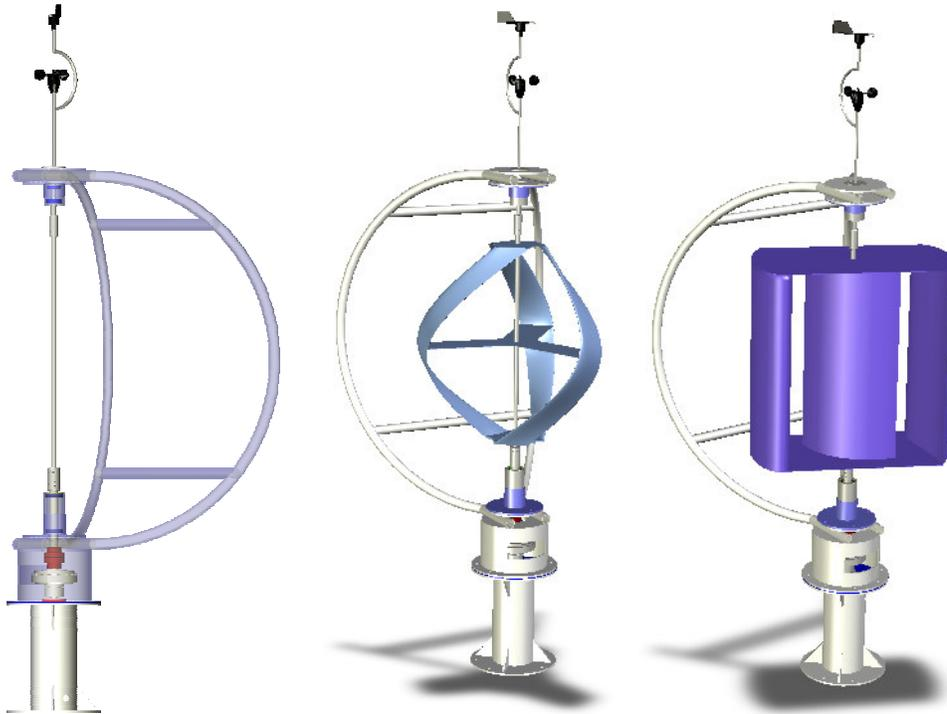
Figure 18. Visualization of the compact version for field tests and demonstration
