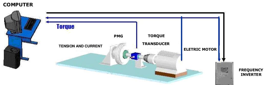
Figure 13. General outline of the generators testing bench
