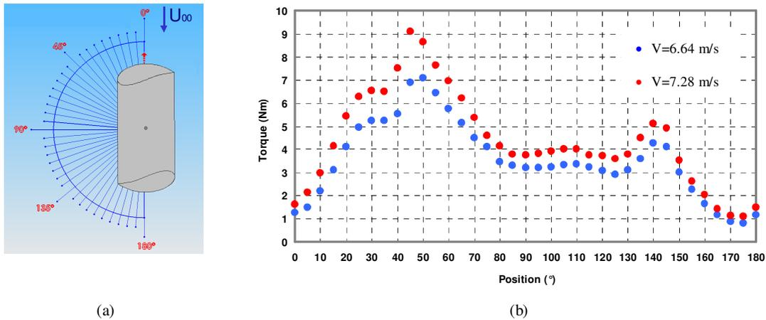
Figure 10. Results of static torque test
