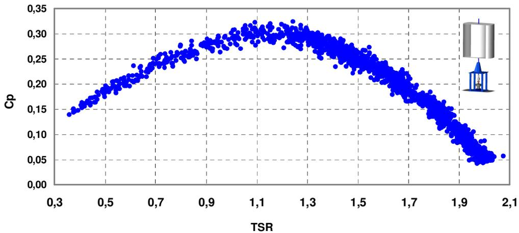
Figure 12. Curve of  $C_p$  versus TSR for the high solidity rotor
