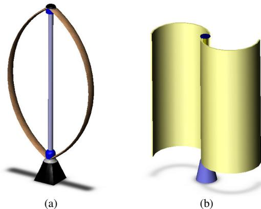
**Figure 1.** VAWT (a) Darrieus concept and (b) Savonius concept
