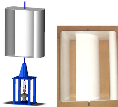
**Figure 6.** Design and prototype of high solidity rotor
