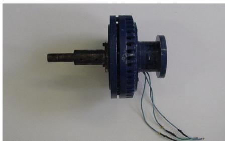
Figure 15. Electric generator E 200W -200
