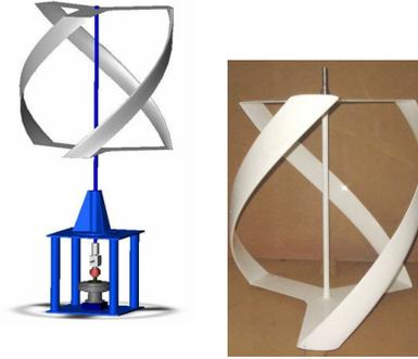
**Figure 5.** Design and prototype of helical rotor with 3 blades
