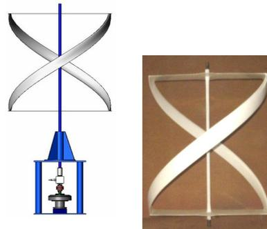
**Figure 3.** Design and prototype of helical rotor with 2 blades
