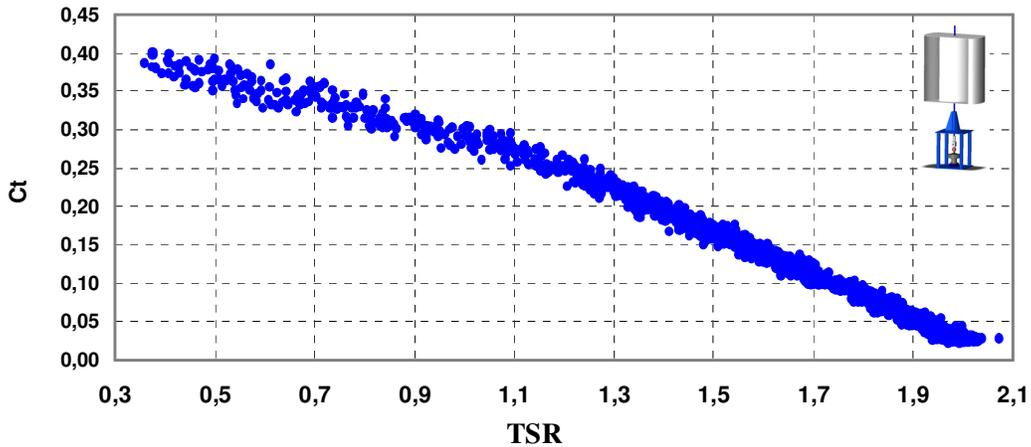
Figure 11. Curve of  $C_t$  versus TSR for the high solidity rotor
