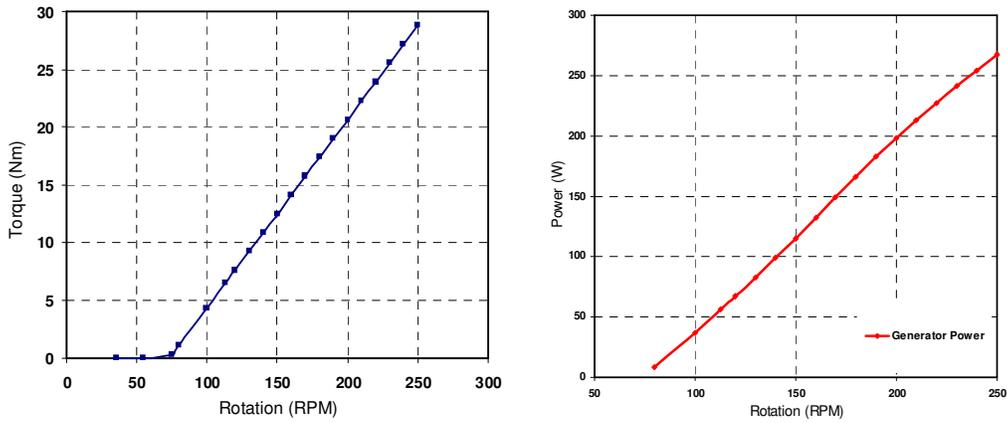
Figure 16. (a) Potency curves with bank of batteries and (b) torque curves with bank of batteries
