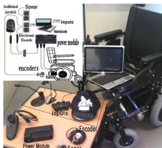
Fig. 1. Hardware Architecture of IntelIWheels.
